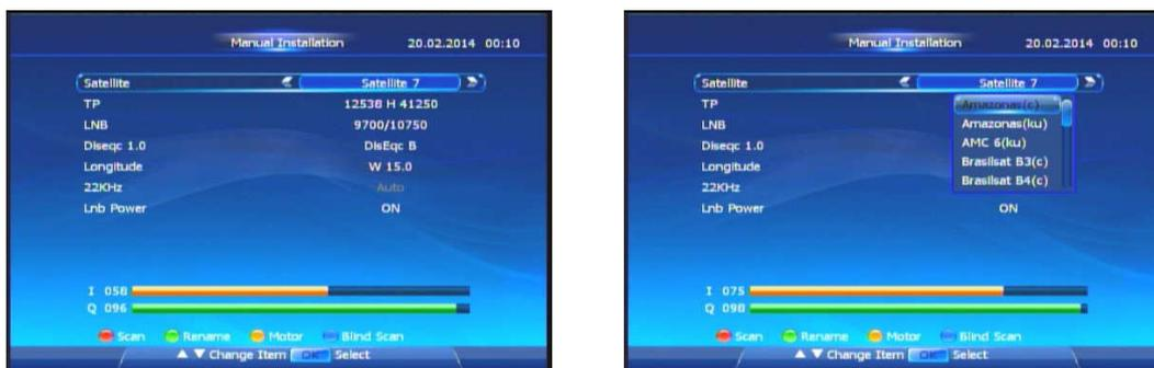
In Blind Installation, you can press **OK** button to show satellite list while focusing first item. Then you can press **▲** or **▼** button to select any satellite you needed.
