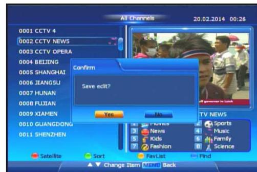
In the Interface of All Channels, you can press ● (yellow) button to call a sub-interface. In this sub-interface, you can mark any channel with a specific tag. After marking, you can sort channels with any one of the eight tags.
