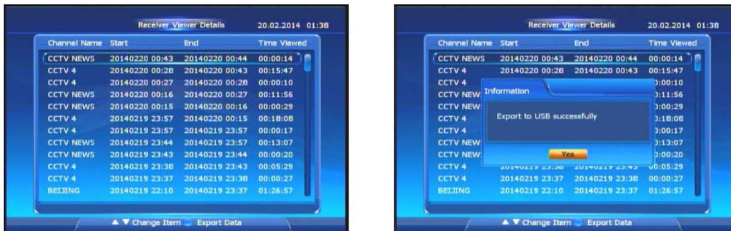
In Receiver Viewer, STB lists all logs of receiving channels including Channel Name, Start-Time, End-Time and Time-Viewed.
