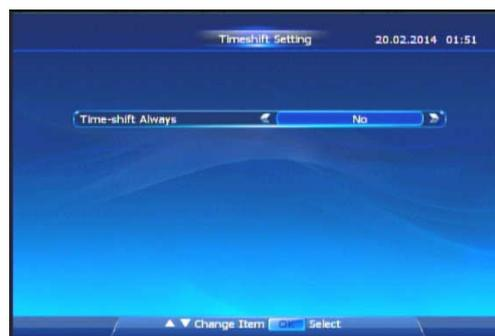
Timeshift Always is “No” by default. While the switch is “Yes”, you can press **FF** or **REW** button to activate Timeshift function without press **PAUSE||** button (need USB Memory disk).
