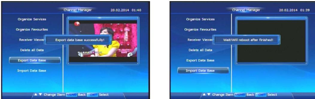
You can export your STB's program database for backup or another STB. Before press OK button, make sure that a USB Memory Disk has inserted into STB. You can import program data using a USB Memory Disk which includes the database file.
